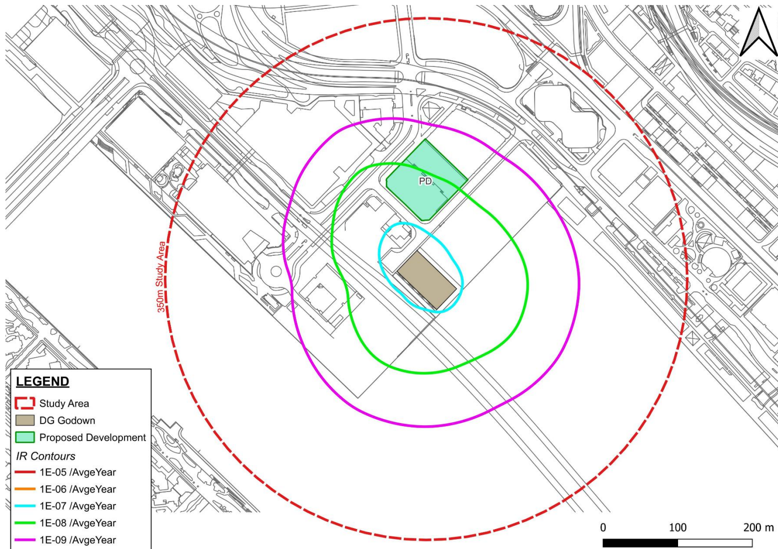
Figure 7 Individual Risk of Kerry DG Godown (Warehouse Fire)
